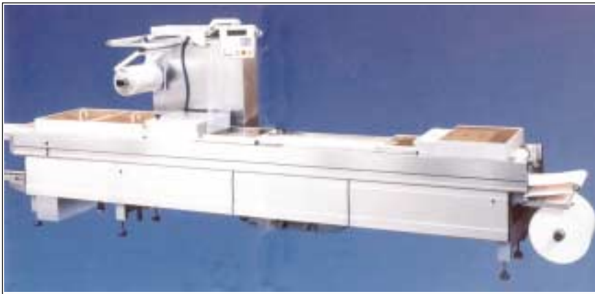
Figure 3: A Swiss Multivac blister-packing machine
